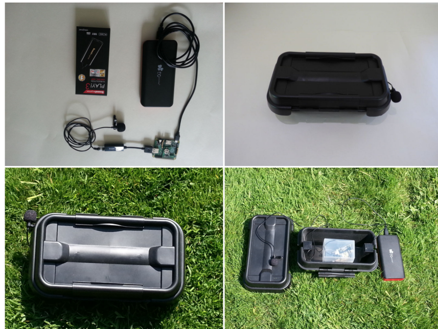
Figure 6. Solo System Audio Recorder with all components and rain-proof box (Whytock, 2018).
